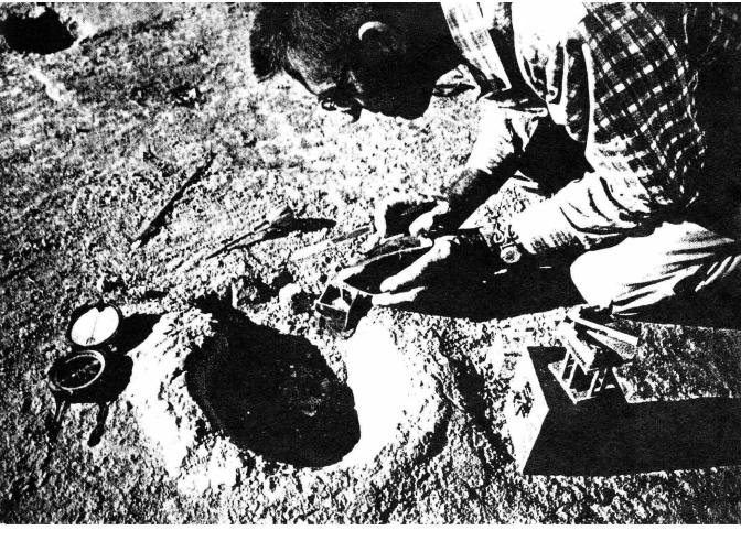
Ancient Hohokam fire pit yields its evidence to Dr. DuBois, one of the world's few specialists in archeomagnetism. He chisels into the fire-hardened clay to isolate a round core, then pours plaster around the sample to protect it, using a brass mold that has been leveled with a spirit level
