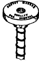
A newly developed survey marker consisting of a corrosion resistant aluminum head threaded to a sharpened carbon steel rod and ribbed for better holding characteristics.
