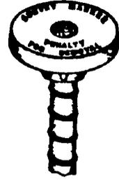
A newly developed survey marker consisting of a corrosion resistant aluminum head threaded to a sharpened carbon steel rod and ribbed for better holding characteristics.
