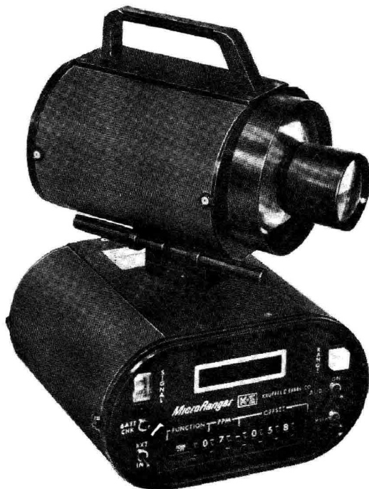
MICRORANGER mounted on transit
