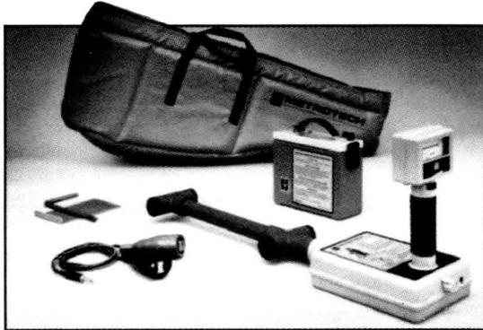
**Passive/Active Locators:** model 650 and 610 feature three selectable frequency ranges, both conductive and inductive coupling, upright operation, push-button depth measurement.
